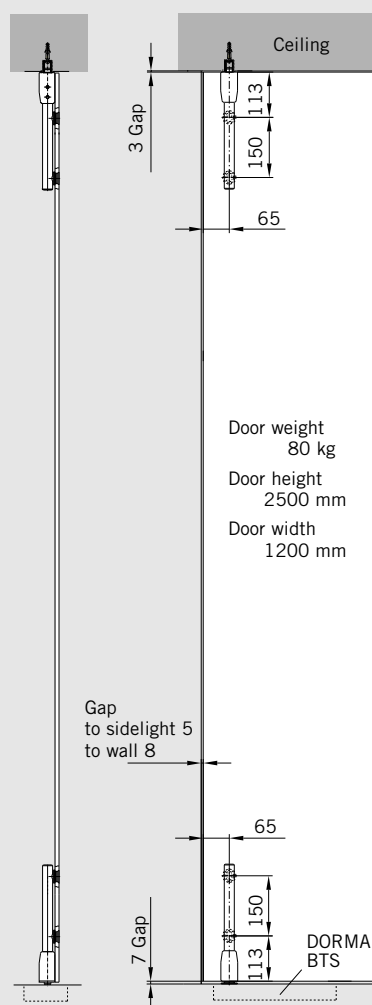
Option: Set 1, but for additional intermediate tube in fixed length for pivot rod pair Intermediate tube in fixed length
