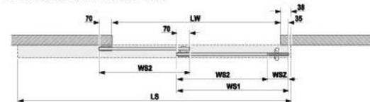
$$WS2 = \frac{LW - WSZ + 70n + 35}{n} \quad WS1 = WS2 + WSZ \quad LS = LW + WS2 + 48 \quad LW = LW - WSZ$$
