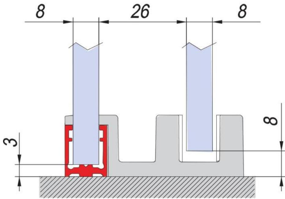
$$\begin{aligned} \text{HM} &= \text{H} - 8 \\ \text{HF} &= \text{H} - 3 \end{aligned}$$
